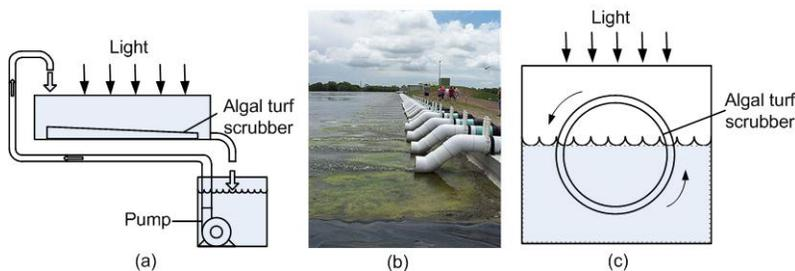
Figure 6. Algal turf scrubber systems (b: courtesy of HydroMentia, Inc.)
