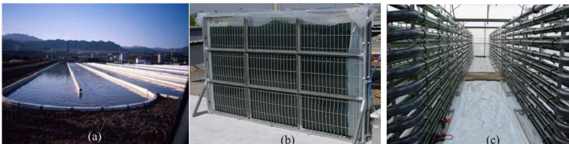
**Figure 4. (a) Raceway pond, (b) plate PBR, (c) tubular PBR (all pictures courtesy of E. M. Grima, University of Almeria, Spain).**
