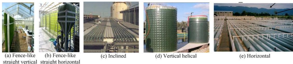
Figure 2. Different designs of tubular PBRs (a and b: courtesy of L. Thomsen, Jacobs University, Germany; c, d, e: courtesy of M. R. Tredici, University of Florence, Italy).
