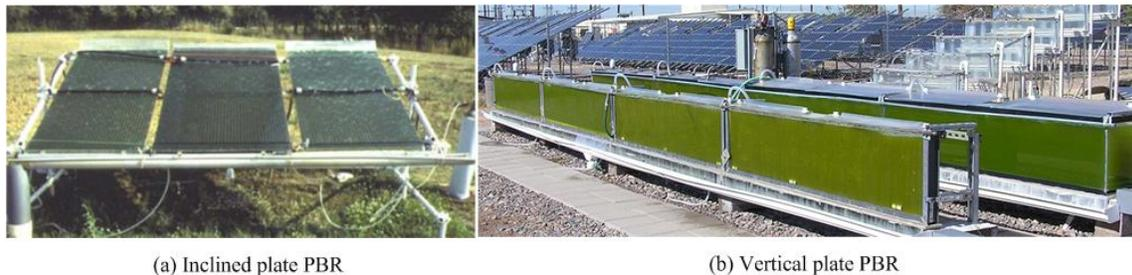
**Figure 3. Two different designs of plate PBRs (a: courtesy of A. Richmond, Ben-Gurion University, Israel; b: courtesy of Q. Hu and M. Sommerfeld, Arizona State University).**
