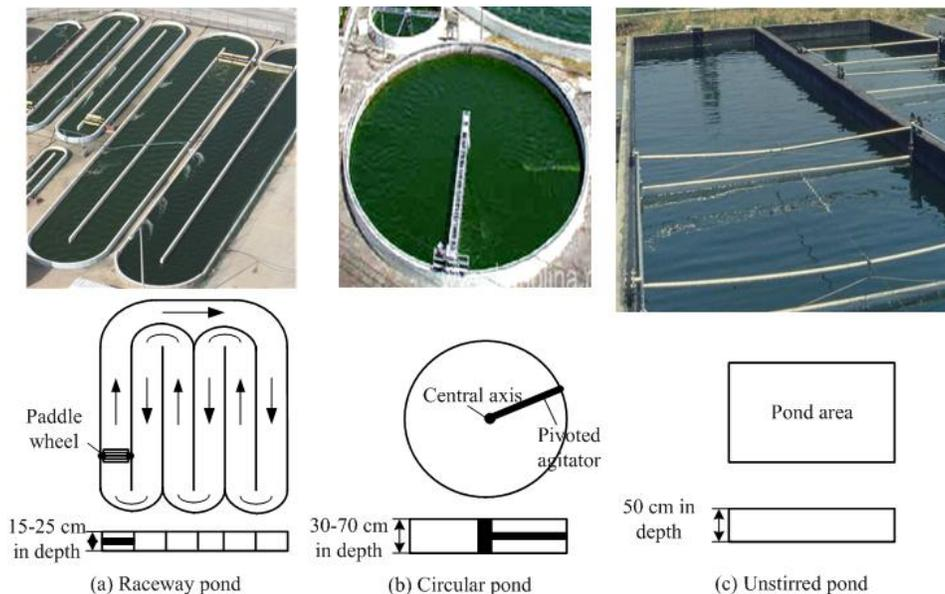
**Figure 1.** Three different designs of open-pond systems (a and b: courtesy of A. Ben-Amotz, National Institute of Oceanography, Israel; c: courtesy of M. R. Tredici, University of Florence, Italy).
